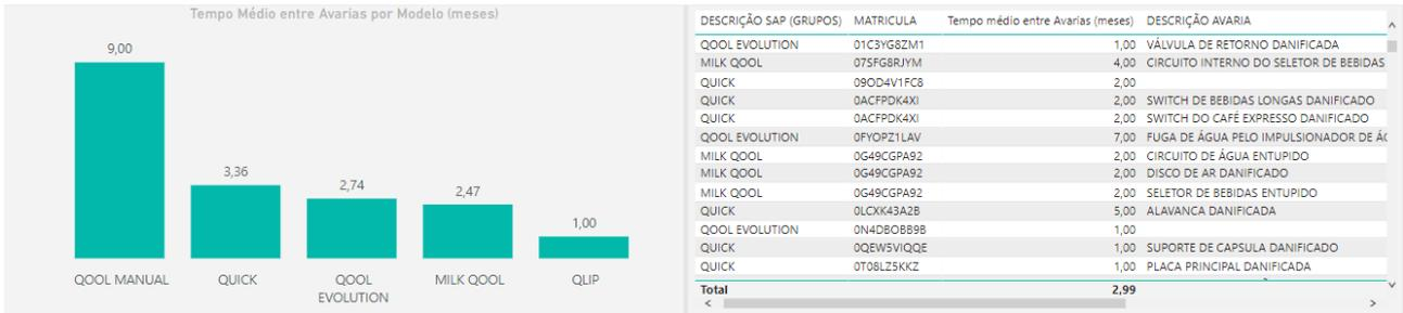
Figure 24 - Average Time Between Failures
