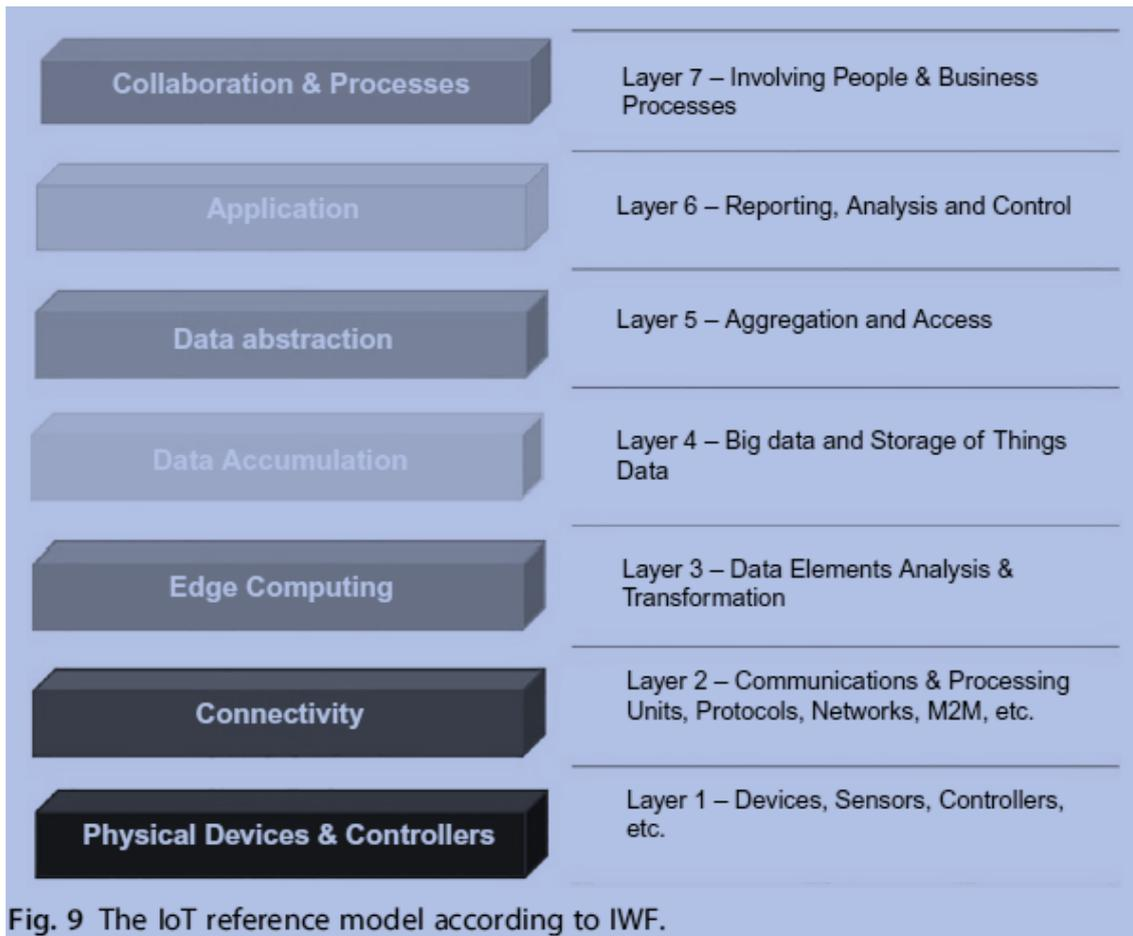
Figure 5- The IoT reference model according to IWF.
