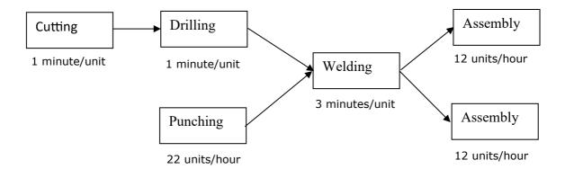
**a)** Cutting: 1 minute/unit or 60 units/hour Drilling: 1 minute/unit or 60 units/hour
