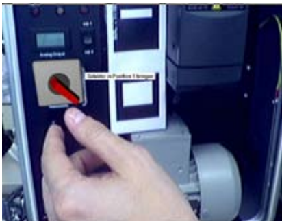
fig. 1: Virtual instruction overlaid onto the command machine
