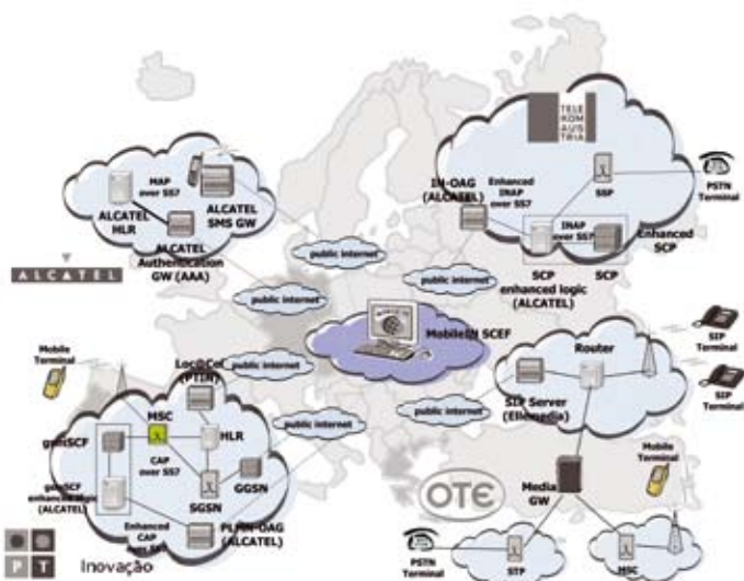
Fig. 1: Mobile IN Architecture and distributed Test-Bed
