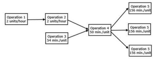
The Operation 3 occurs separately from, and simultaneously with, the Operation 1 and Operation 2. The product only needs to go through one of the three final operations (Operation 5), since they are in parallel. Assume that the company works 8 hours per day, the yield in each phase is 100%, there are no stoppages, and stock cannot be accumulated between the different operations of the process.
